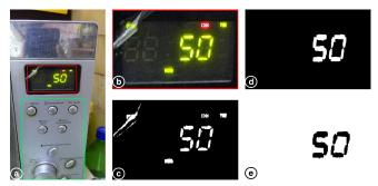
Figure 13. VizLens::LCD Display Reader applies OCR to recognize digits on the portion of the interface that is an LCD screen. (a) Separated dynamic and static regions. (b) Image sharpening using unsharp masking. (c) Intensity-based thresholding. (d) Morphological filtering and small blob elimination. (e) Selective color inversion.
