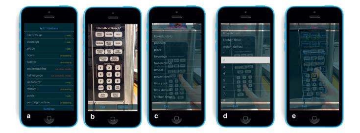
Figure 2. VizLens mobile app interfaces. (a) App's main screen, listing all available interfaces and status, as well as Add Interface and Settings options. (b) Interface for Add Interface, where the user can take a photo and denote a name for it. (c) When user selects an interface, he can start to get feedback. (d) When selecting a visual element, the app start providing guidance. (e) a virtual interface layout that users can explore directly on the touchscreen.
