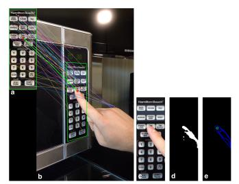
Figure 4. Real-time recognition and control using VizLens. Recognition result, showing (a) reference image and (b) input image. (c) Input image warped to reference image's frame allowing the coordinates of the elements previously labeled to be retrieved. (d) Result of skin color thresholding, and (e) calculated fingertip location.
