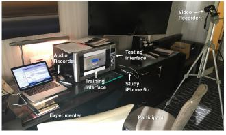
Figure 6. User study setup. A printer's interface is printed out on paper and used for training. The microwave interface was used for controlled testing, followed by more exploratory use of other interfaces nearby (*e.g.*, remote control, thermostat, vending machine). The study was conducted in a hotel room and was video and audio recorded.
