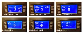
Figure 12. VizLens::State Detection detects screen state and adapts to it. In this example, VizLens figures out which of six states this fancy coffee machine is in, and provides feedback or guidance specific to that screen.
